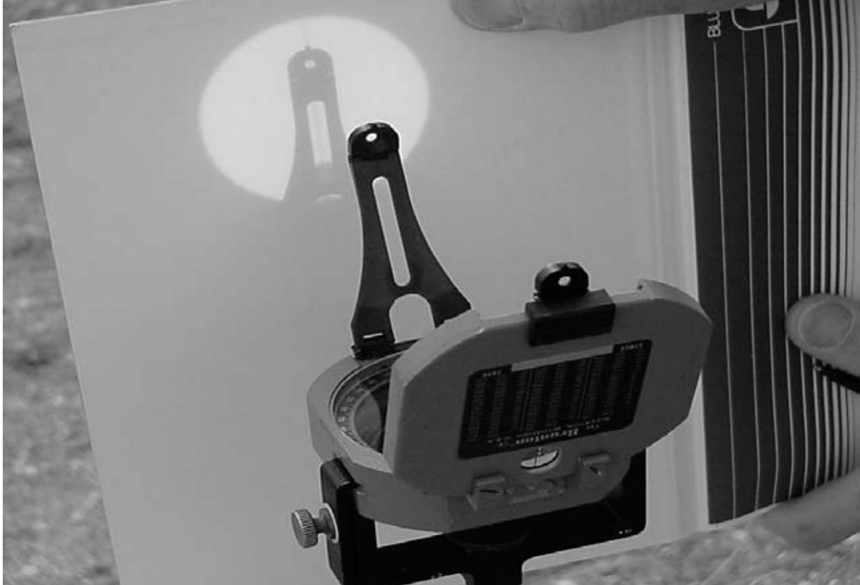
Figure 3: Measuring the Sun's azimuth. Ensure that the black line's reflection is centered on the cross hairs in the reflection. Taken from Figure 2.16 of EPA-454/B-08-002.
