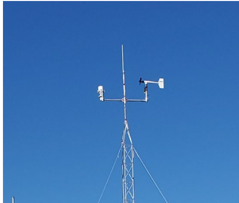
Figure 9: Example of wind speed and direction sensor
