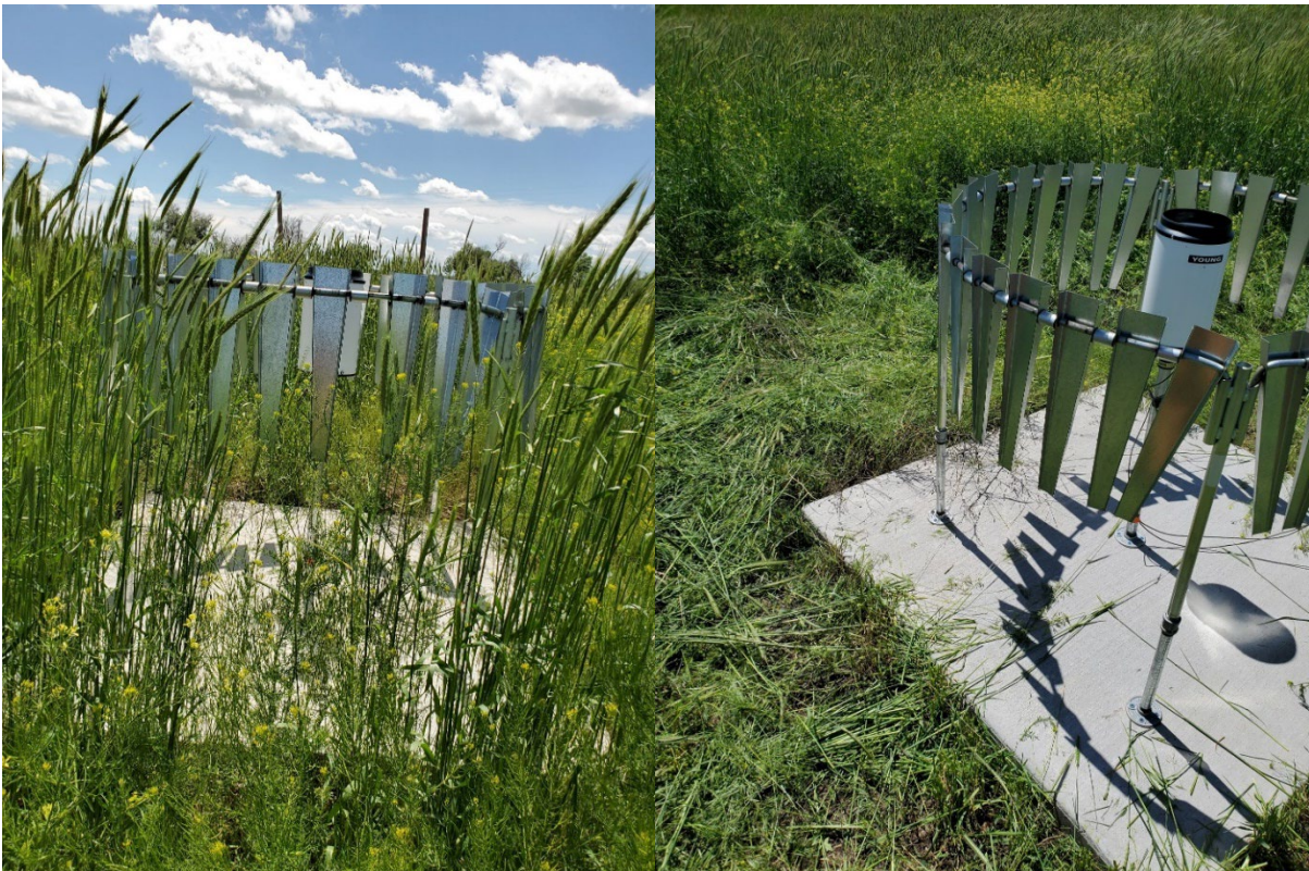
Figure 16: Left) Example of tall vegetation that should be removed. Note that vegetation is taller than the height of the wind screen. Right) Example of cleared vegetation. Note, this is the Weld Operated Precipitation Equipment.
