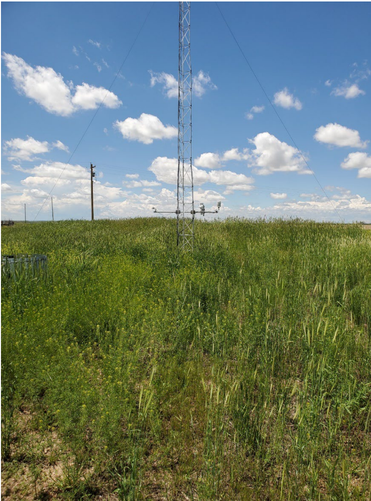
Figure 20: Example of tall overgrowth near tower
