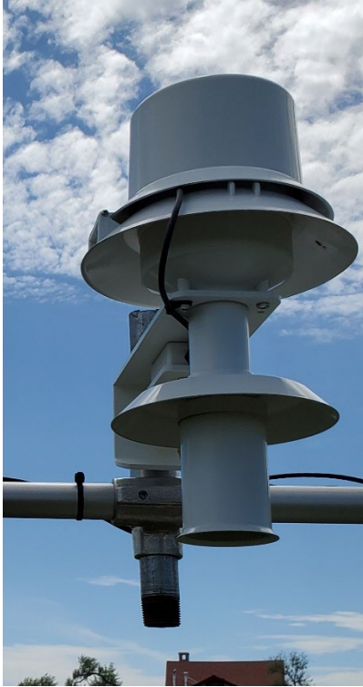
Figure 10: Example of temperature sensor
