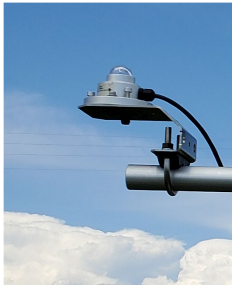
Figure 8: Example of solar radiation sensor
